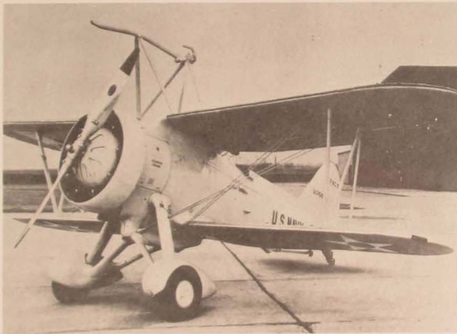
U.S. experimentation with the piggy-back concept dates to the 1920s, when the Sperry Messenger, (shown above during two stages of restoration) was tested at McCook Field, Ohio. The hook on the top wing engaged a trapeze grappling apparatus hanging from an airship. . . . In the early 1930s the Navy's Sparrow Hawks (right) attached to the dirigibles USS Macon and Akron, three of them being destroyed in the Macon disaster on 12 February 1935.
